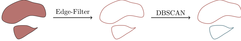
Fig. 18: The postprocessing pipeline for the panoptic-segmentation. The panoptic-segmentation is at first edge filtered, drastically reducing the points in a cloud, only leaving the enclosing points of an instance (may it be a thing or stuff). Then the DBSCAN algorithm is applied to all the different thing and stuff instances in the image to separate instances of the same class that have a margin in between them. After the DBSCAN algorithm, we extract the convex hull from the points, being our polygon for further analysis.
