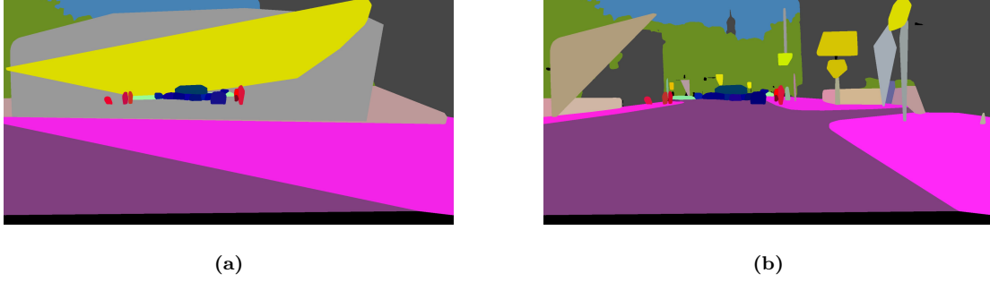
Fig. 17: The input to the algorithm is the panoptic-segmentation of fig. 16 (b) . On the left-hand side, only the convex hull is formed, while on the right-hand side we applied the edge filtering and the DBSCAN algorithm as well as thresholding the minimum allowed area. In both cases we used the plain panoptic-segmentation for classes that are of no interest for the later analysis of pedestrian crossings ( sec. 7 ), e.g. sky, vegetation and buildings. One can see the problems, if DBSCAN is not applied, with instances leaking over other instances and outliers, drastically enlarging instances when the convex hull is formed (a).
